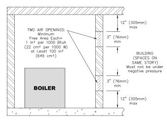
Figure 1.1: Air Openings – All Air from Indoors on the Same Floor
